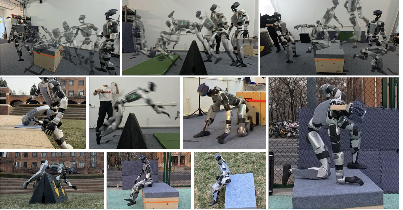
Fig. 1: Deep Whole-Body Parkour. Our framework enables a humanoid robot to autonomously traverse challenging obstacles that impose strict geometric constraints on robot odometry. The top row visualizes the dynamic execution of vaulting, diving, and jumping using stroboscopic photography. The bottom rows demonstrate the policy’s robustness in diverse indoor and outdoor environments. Crucially, the system utilizes onboard perception to proactively adjust its approach trajectory, ensuring precise foot placement and hand contact for successful whole-body interaction. Please visit the project website and see the open-sourced infrastructure at https://project-instant.github.io/deep-whole-body-parkour
